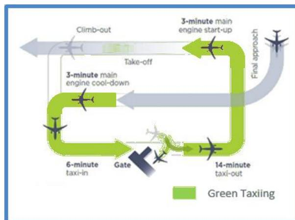
Figure 12: non-autonomous solutions footprint during LTO cycle.
