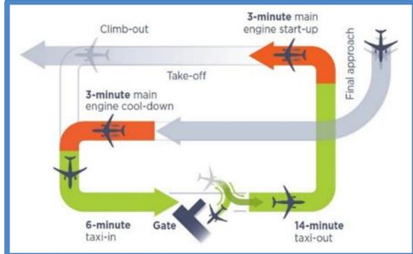
Figure 10: LTO cycle for e-taxi systems installed on the main landing gear.
