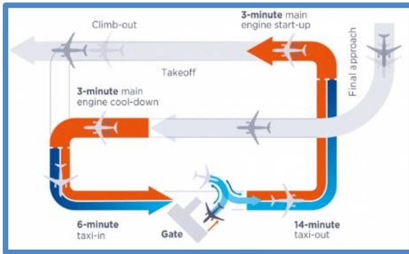
Figure 9: LTO cycle for hybrid operation (SET/e-taxi).
