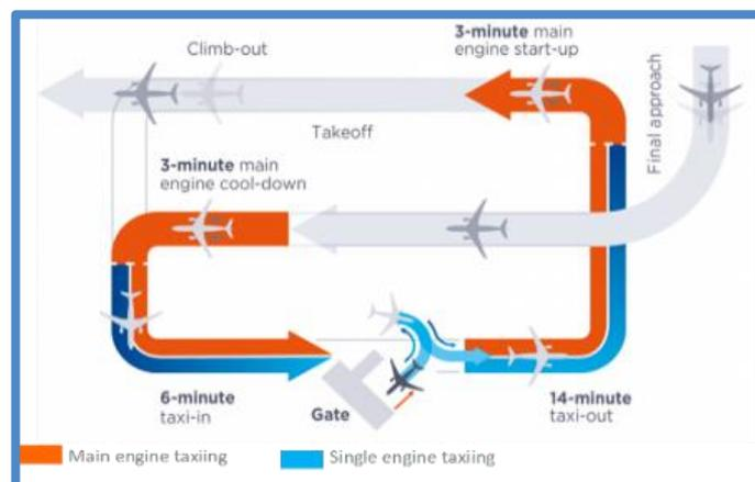
Figure 6: Single Engine-off footprint during LTO
