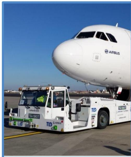
Figure 11. Towing vehicle coupled to an aircraft.
