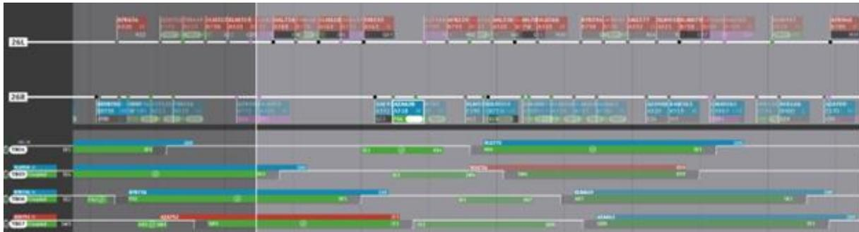
**Figure 13: Supervision HMI with arriving and departing aircraft on the top and the tugs underneath with allocations.**
