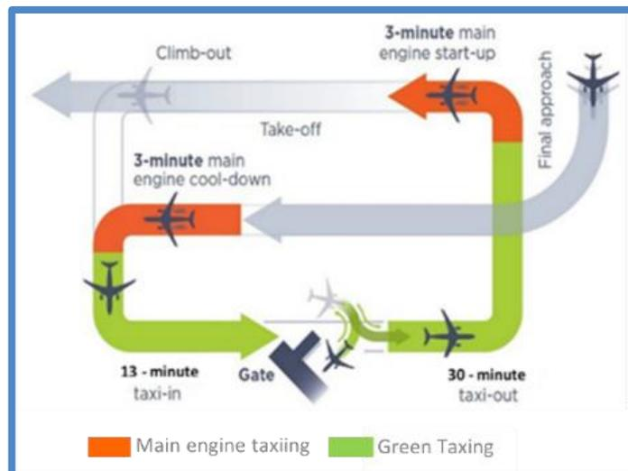
**Figure 8: LTO cycle for e-taxi systems installed on the nose landing gear.**
