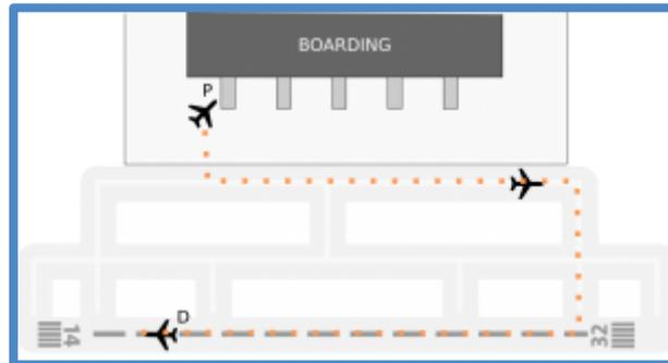
Figure 3: EXOT time calculation methodology
