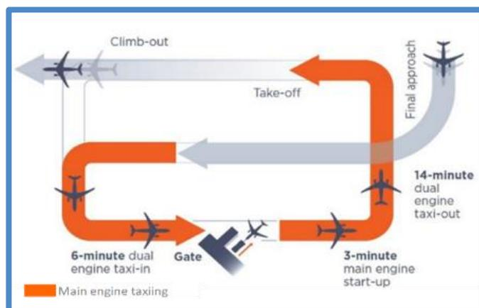
Figure 5: Main Engine-on footprint during LTO
