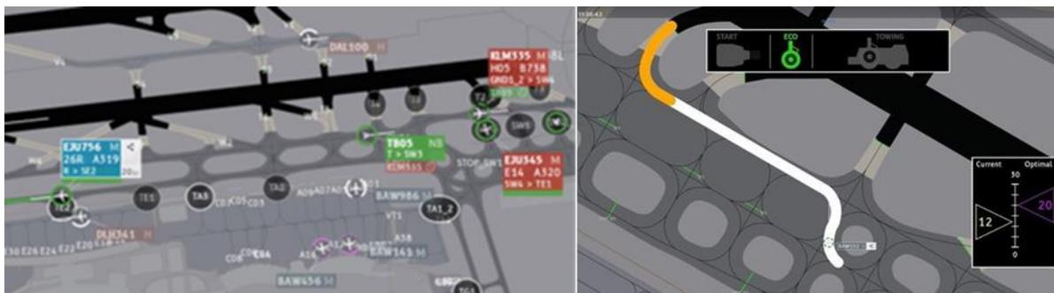
Figure 15: Left: Portion of the radar image representing aircraft, their taxiing techniques, and the towing vehicles.
