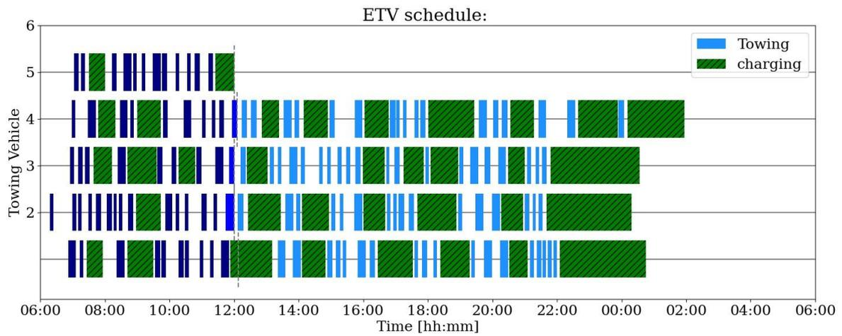
Figure 6: tug allocation at 2 PM, after tug 5 has been sent to maintenance
