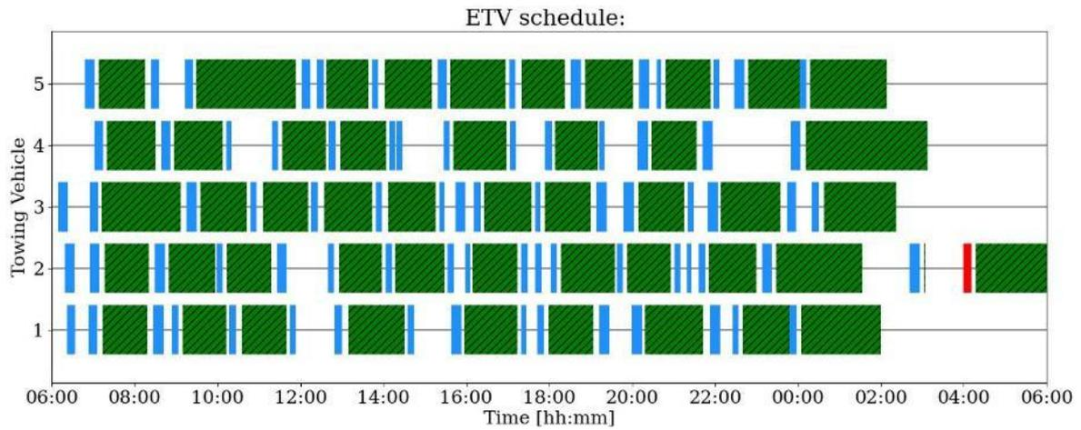
Figure 10: Tug allocation after a manual flight reassignment by the TFM (in red).
