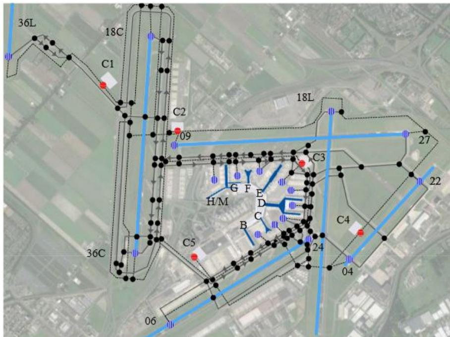
**Figure 3** EHAM road network. The runways and piers are displayed in blue, the taxiway in solid lines, and the service road network in dashed lines. Black circles indicated junctions, vertically hatched circles indicate gate/runway access points, and red circles indicate possible charging station locations. The tug depot is located at C5.
