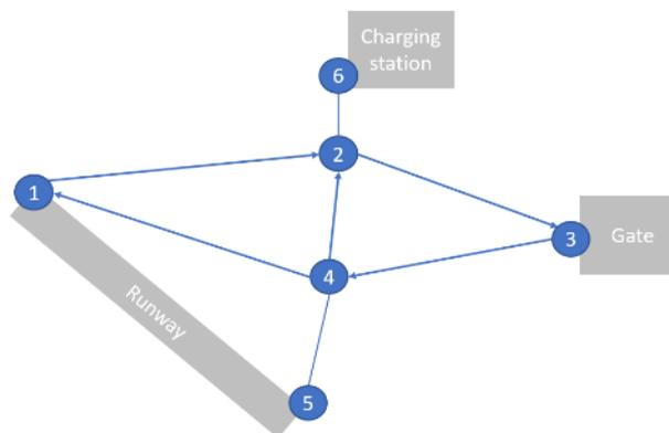
**Figure 2: Mock airport road network. The taxiway network, connects the gates, runways, and tug charging stations with each other.**
