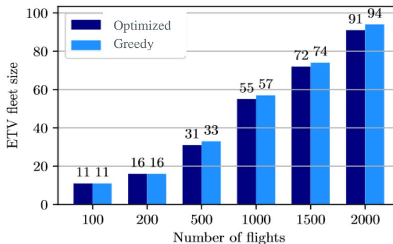
**Figure 11: Number of vehicles required to tow all aircraft using the greedy AEON solution and a linear programming formulation.**
