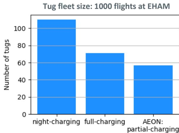
Figure 12: Required fleet sizes using different charging protocols [4].
