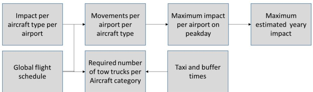
Figure 2: Calculating maximum total impact of introducing towing
