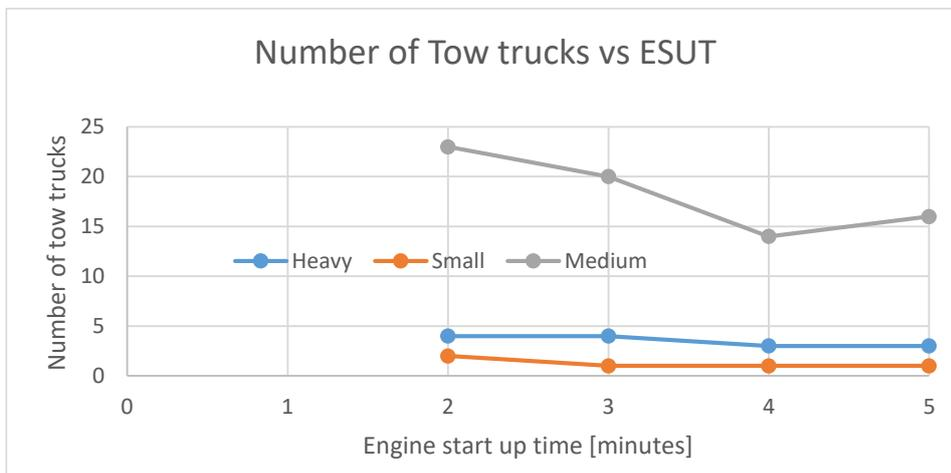
Figure 14: Impact of engine start up time on number of tow trucks deployed
