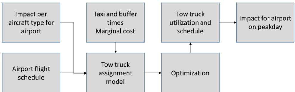
Figure 3: Optimizing Tow truck assignment workflow
