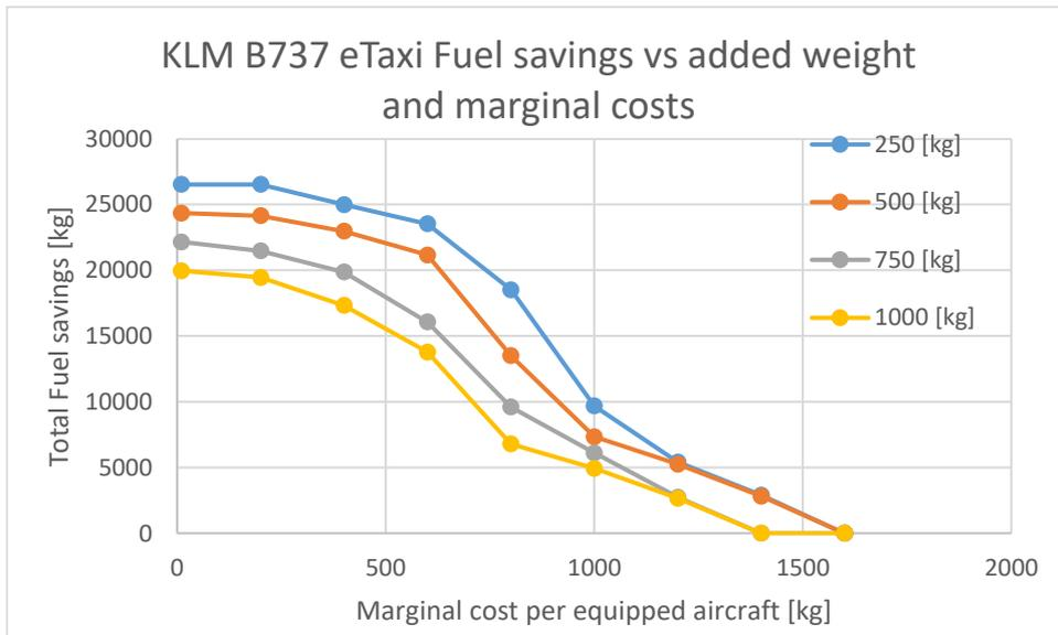
Figure 45 : Impact of weight and marginal cost on fuel savings per peak day on KLM 737 aircraft
