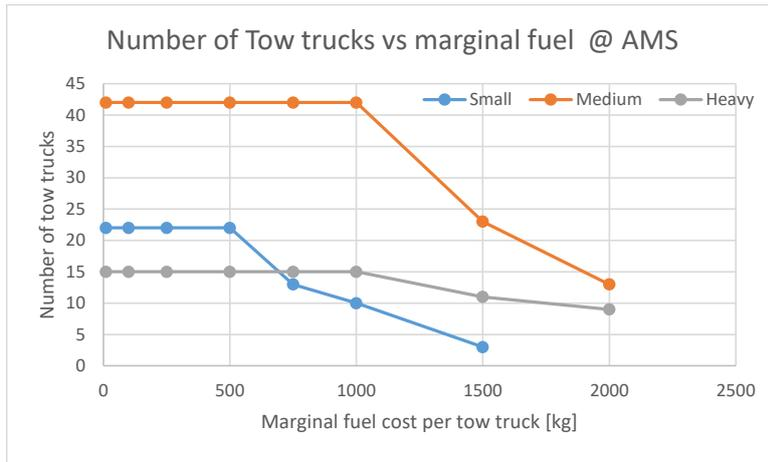
Figure 5: Number of trucks deployed vs. marginal fuel cost per truck on a peak day @ AMS
