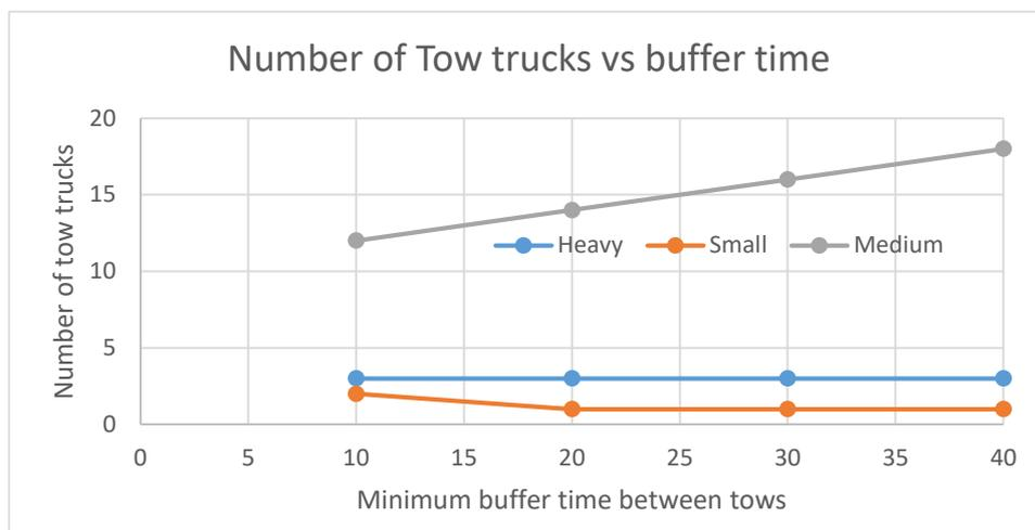
Figure 12: Impact of buffer time on number of tow trucks required
