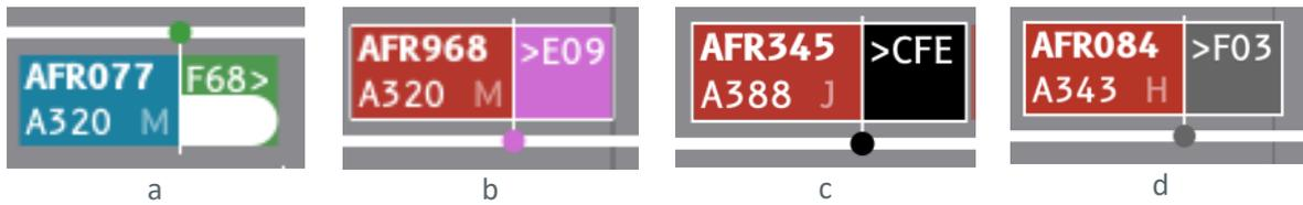
Figure 7: Aircraft's labels on the runway's timeline indicating the chosen taxiing technique. Taxibot (a), Electric taxiing (b), Full Engine Taxiing (c), Single Engine Taxiing (d).
