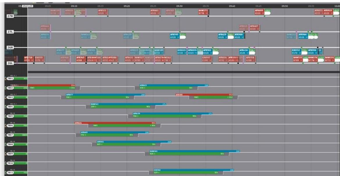
Figure 3: Supervision HMI with arriving and departing aircraft on the top and the available tugs underneath.
