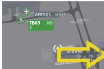
Figure 25: Arrow on the border of the window of the A-SMGCS to indicate that the BAW141 is on the right.
