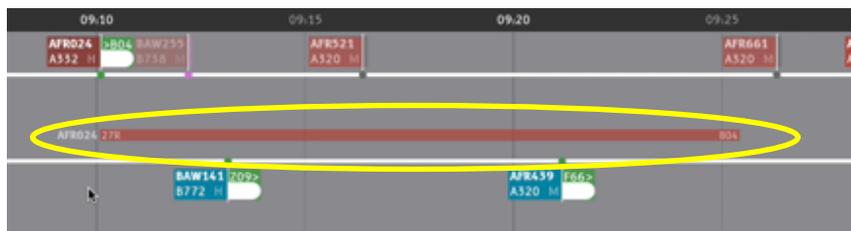
Figure 20: the ghost label (surrounded in yellow) corresponding to the flight AFR024 appears near the mouse cursor during the drag.
