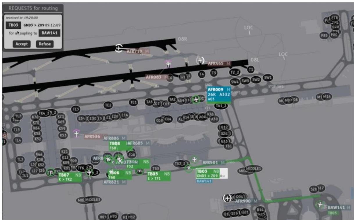
Figure 28: The request route is displayed from current position of the TB03 to coupling position
