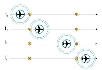
Figure 6: Calculated time points  $t_1$ ,  $t_2$ ,  $t_3$ , and  $t_4$  relative to each edge on an agent's route. Inner circle represents area of agent with radius  $r_{a_i}$ , middle circle has radius  $r_{a_i} + r_{a_j}$  representing the area of both agents, and outer dashed circle represents the combined shape with radius  $r_s$ .
