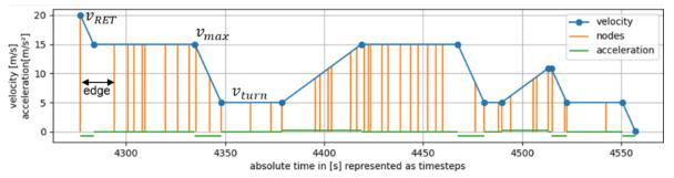
Figure 1: Exemplary velocity profile of the route of a landing aircraft. Orange lines: junction points in taxiway network (nodes). Vehicles travel along centrelines (edges).
