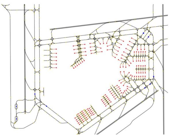
Figure 4: Part of the graph representation of Amsterdam Airport Schiphol. Taxiway edges (black), taxiway nodes (yellow), ramp nodes and edges (red), decoupling nodes (blue), and runways (grey)
