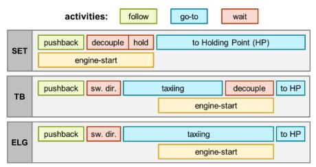
Figure 2: Exemplary activity sequence for different taxiing techniques of an outbound aircraft. "sw. dir.": switch direction
