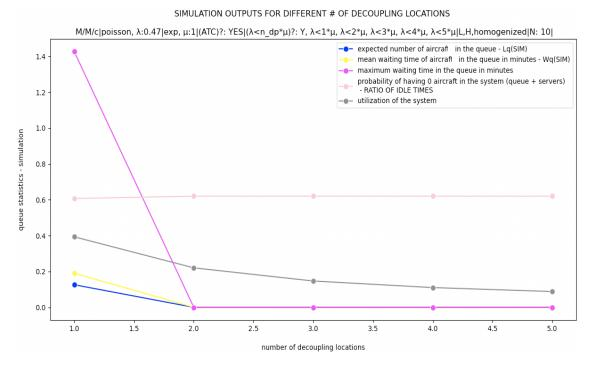
Figure 19 : Simulation outputs for M/M/c|poisson,  $\lambda$ :0.47|exp,  $\mu$ :1|(ATC)?: YES|( $\lambda$ <n\_dp\* $\mu$ )?: Y,  $\lambda$ < $\mu$ ,  $\lambda$ <2 $\mu$ ,  $\lambda$ <3 $\mu$ ,  $\lambda$ <4 $\mu$ ,  $\lambda$ <5 $\mu$ |L,H,homogenized|N=10|
