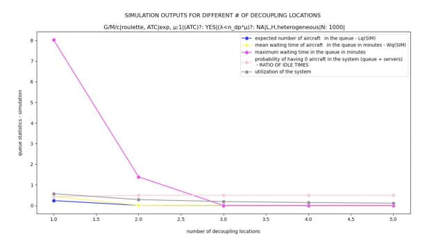
Figure 30 : Simulation outputs for G/M/c|roulette, ATC|exp,  $\mu$ :1|(ATC)?:YES|( $\lambda$ <n\_dp\* $\mu$ )?:NA|L,H, heterogeneous|N=1000|
