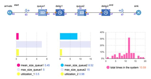
Figure 40: Two sequential queues with arrival/service1/service2 rates of 1/2/1 – simulation state at 63<sup>rd</sup> arrival
