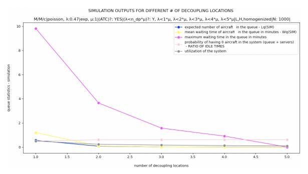
**Figure 21 :** Simulation outputs for M/M/c|poisson,  $\lambda$ :0.47|exp,  $\mu$ :1|(ATC)?: YES|( $\lambda$ <n\_dp\* $\mu$ )?: Y,  $\lambda$ < $\mu$ ,  $\lambda$ <2 $\mu$ ,  $\lambda$ <3 $\mu$ ,  $\lambda$ <4 $\mu$ ,  $\lambda$ <5 $\mu$ |L,H,homogenized|N=1000|
