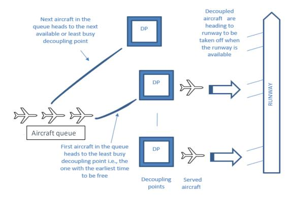
Figure 17: Representation of single queue multiple parallel decoupling locations
