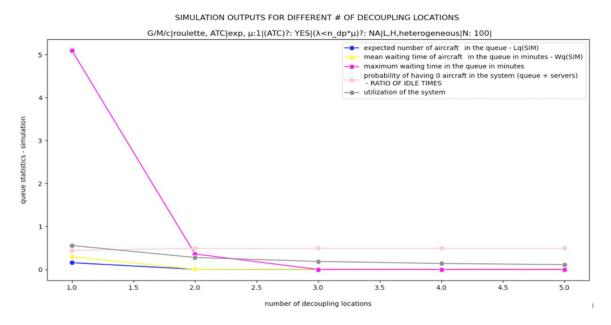
**Figure 29 : Simulation outputs for** G/M/c|roulette, ATC|exp,  $\mu$ :1|(ATC)?:YES|( $\lambda$ <n\_dp\* $\mu$ )?:NA|L,H, heterogeneous|N=100|
