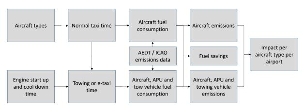
Figure 1: Calculation for determining impact numbers per aircraft type and airport
