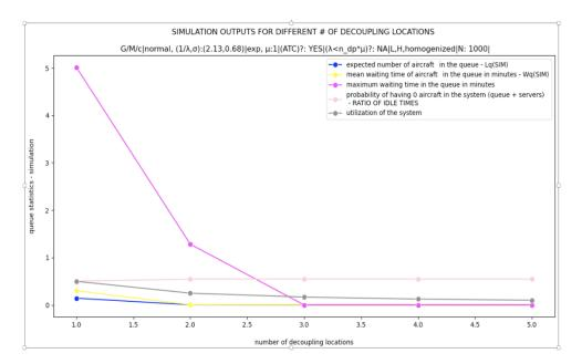
Figure 36 : Simulation outputs for G/M/c|normal,(1/ $\lambda$ ,\sigma):(2.13,0.68)|exp,µ:1|(ATC)?:YES|( $\lambda$ < n\_dp\*µ) ?:NA|L,H,homogenized |N=1000|
