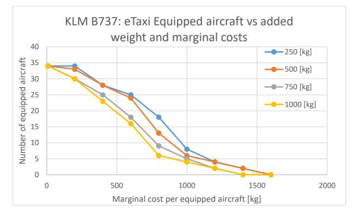
Figure 44: Impact of weight and marginal cost on the number of KLM 737 aircraft equipped
