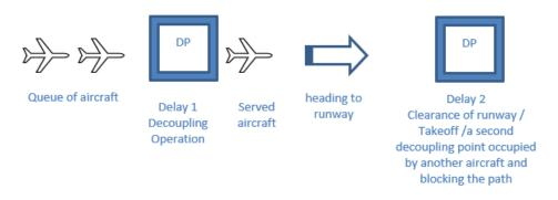
Figure 18 : Representation of an example of sequential delay locations
