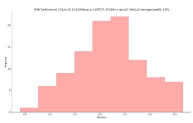
**Figure 32 :** Interarrival times of aircraft for G/M/c|normal,( $1/\lambda,\sigma$ ):(2.13,0.68)|exp,µ:1 |(ATC)?:YES| ( $\lambda$ < n\_dp\*µ) ? : NA |L,H,homogenized |N=100|
