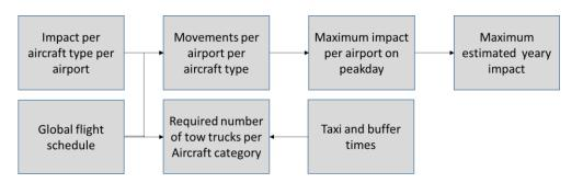
Figure 2: Calculating maximum total impact of introducing towing
