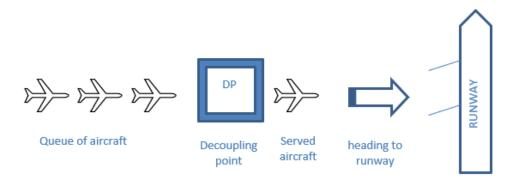
Figure 16: Representation of single queue single decoupling location
