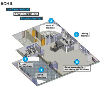
Figure 2: ACHIL simulation facilities
