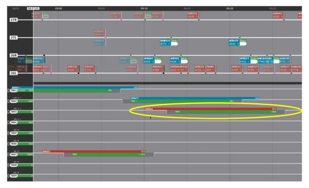
Figure 21: the flight AFR024 has been affected to the tug TB03 (circled in yellow).
