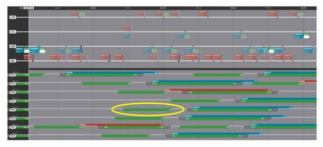
Figure 29: Supervision tool with additional elements indicating the taxiing between the decoupling point from its previous mission and the coupling point of the following one.
