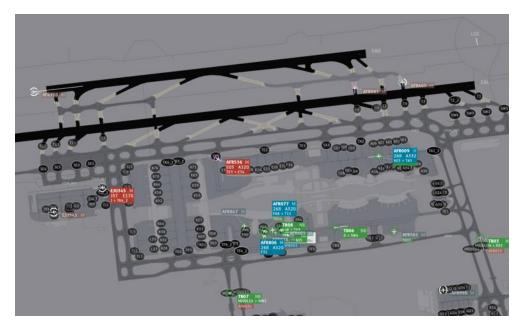
Figure 14: A-SMGCS HMI used by the TFM position
