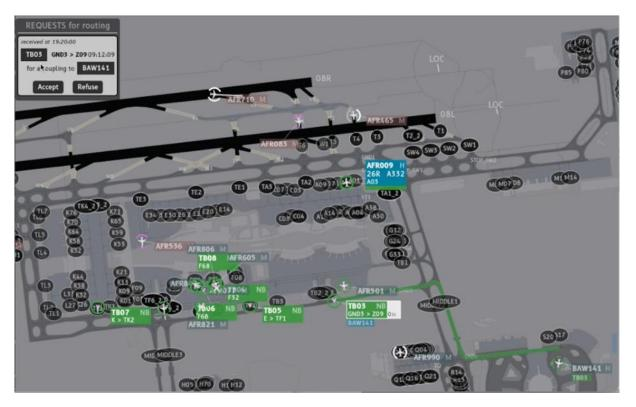
Figure 28: The request route is displayed from current position of the TB03 to coupling position
